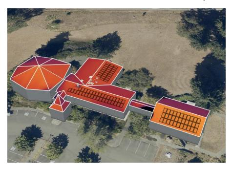
3 FranklinWh aPower 2 batteries will have Capacity of 45kWh. These will be used to power lights and the refrigerators during a power outage. The batteries are 45x29" in size and will be installed outside the church building.
